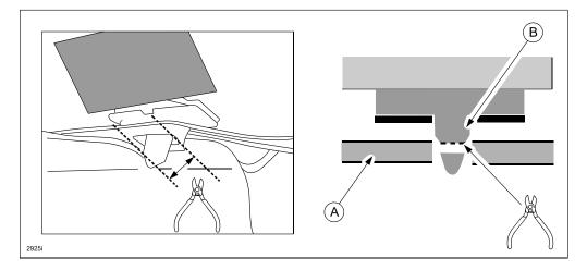
f. Pull down the reinforcement panel by the masking tape (A) using a suitable tool (B), such as a retaining clip remover, to provide clearance between the reinforcement panel and the remainder of the cut pin. Make sure there is no remaining contact between the pin and the reinforcement panel.
