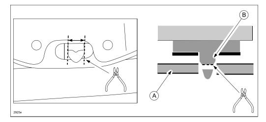
Pull down the reinforcement panel by the masking tape (A) using a suitable tool (B), such as a retaining clip remover, to provide clearance between the reinforcement panel and the remainder of the cut pin. Make sure there is no remaining contact between the pin and the reinforcement panel.
