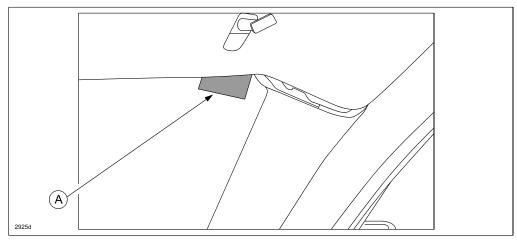
f. Gently pull down on the headliner to provide enough space to insert the side cutters.
