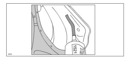
5. Allow the bond to dry until it's surface does not stick to finger.
