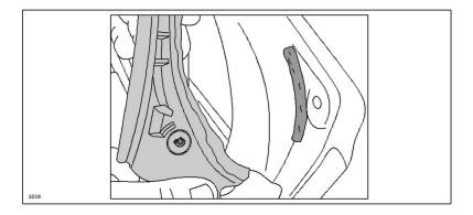
6. Install the weatherstrip to the door panel and press on the bonding area (A).
