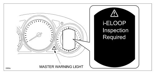
c. DTC P1794:00 (Capacitor (i-ELOOP) system: Capacitor (i-ELOOP) malfunction) is stored in PCM memory. Customers having this concern should have their vehicle repaired using the following repair procedure.
