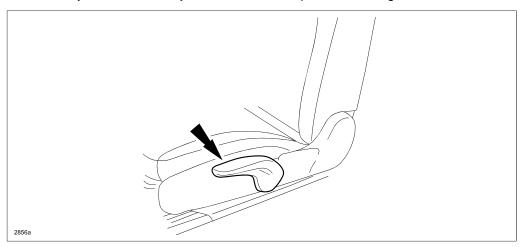
This may be caused by a broken front seat side cover that interferes with the operation of the seat lifter mechanism. The cover may have been previously broken by an outside impact.
