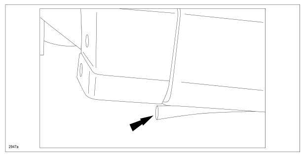
This concern may occur when the vehicle is driven in freezing temperatures. Snow and moisture adhere and freeze onto the rubber protector and when the door is opened, the rubber protector can tear or stretch, coming off the fasteners.
