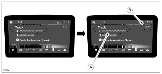
Symptom 2: The track list does not open after inserting the CD, but the "Disc loading" appears on the display. This is caused by improper software of the CD player. The software of CD player has now been changed to correct this issue.
