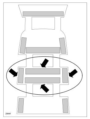
4. Press the two (2) seat warmer bridges (A) into the groove in the pad.
