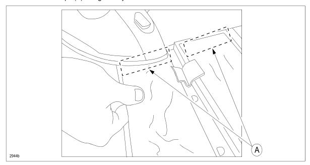
**NOTE:** DO NOT apply the iron directly to the cushion pad, as it could melt the pad.
