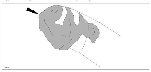
2. Apply the grease all the way around the inner ball joint edge.
