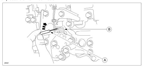
b. Remove oil pressure switch B.
