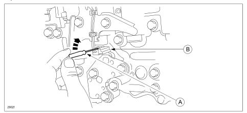
b. Remove oil pressure switch B.
