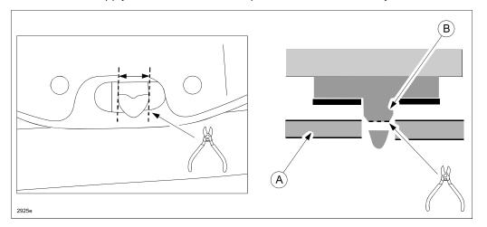
h. Pull down the reinforcement panel by the masking tape (A) using a suitable tool (B), such as a retaining clip remover, to provide clearance between the reinforcement panel and the remainder of the cut pin. Make sure there is no remaining contact between the pin and the reinforcement panel.
