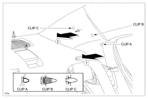
b. Remove the clips (A) securing the headliner to the roof panel.
