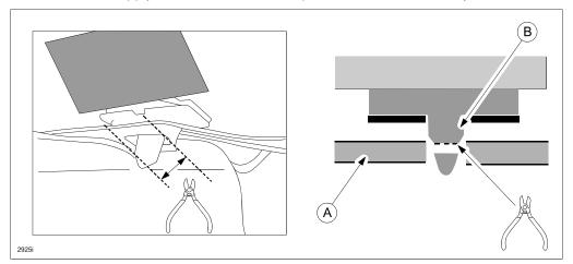
f. Pull down the reinforcement panel by the masking tape (A) using a suitable tool (B), such as a retaining clip remover, to provide clearance between the reinforcement panel and the remainder of the cut pin. Make sure there is no remaining contact between the pin and the reinforcement panel.
