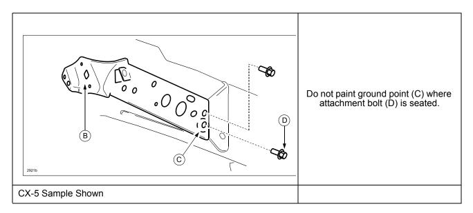
Customers concern can be resolved by sanding off paint at ground point (C) where attachment bolt (D) is seated. After installing the bolt (D), apply touch-up paint to the exposed base material area of the front fender stay.
