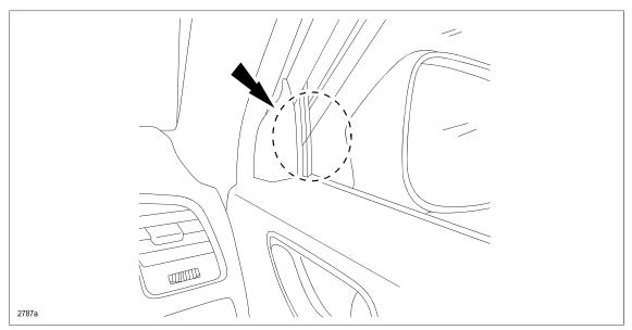
The rattle noise may be caused by insufficient glass run channel holding force. To eliminate this concern, the shape of glass run channel has been changed in order to increase the holding force.
