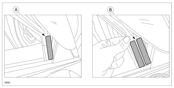
8. Apply an adhesion promoter (one that is suitable for use on plastic) to the three (3) locations where the pads will be attached.
