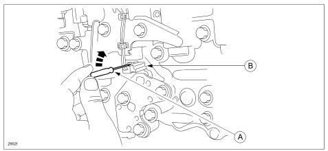
b. Remove oil pressure switch B.
