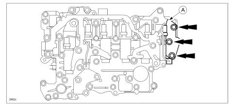
c. Detach the tab shown and remove oil pressure switch A from the control valve body.
