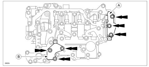
10. Connect the oil pressure switches A and B connectors.
