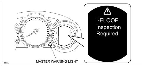
c. DTC P1794:00 (Capacitor (i-ELOOP) system: Capacitor (i-ELOOP) malfunction) will be stored in PCM memory.
