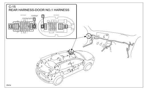
The symptoms listed above may be caused by corrosion of the C-15 connector terminals due to water intrusion through the front door. In low ambient temperatures, the door harness hardens. If the door is fully opened, it may create a gap between the door and the door harness grommet, which may allow water to enter through the gap.
