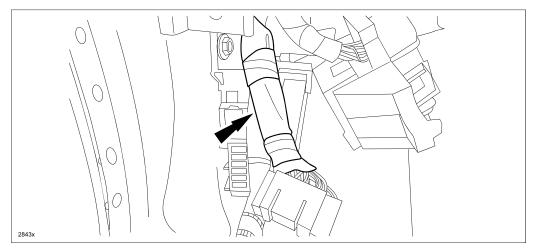
32. Pull out the C-15 connector from the front pillar to the door side.
