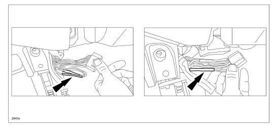
30. Wrap the harness with electrical tape as shown below.
