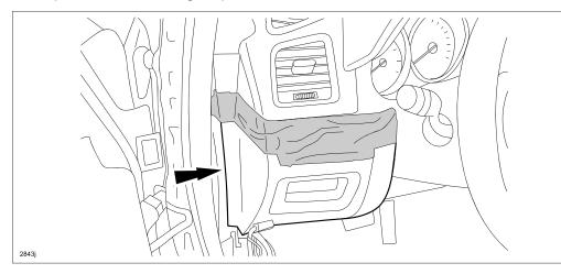
17. Pull the C-15 connector out of the front pillar inside the cabin.
