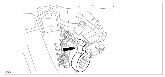
31. Install the protector tube as shown below, then secure both ends with electrical tape.
