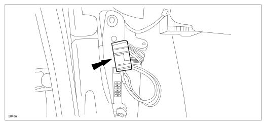
29. Bend the excess length of wires (as shown below) to match with the other wires.
