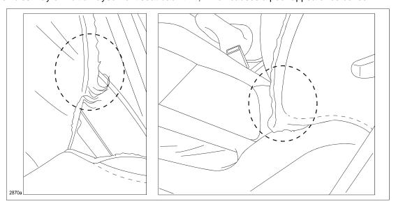
This may occur under special conditions where the customer rubs against the seat back trim when entering or exiting the vehicle. If the customer wears clothes designed with metal accessories (i.e. jewelry, tack, zipper or Velcro), the damage may occur.
