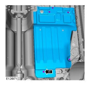
17. Remove the retaining bolt.
