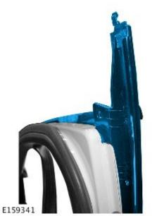
**12.** Check the door seam condition (incorrect (gap) seam shown).
