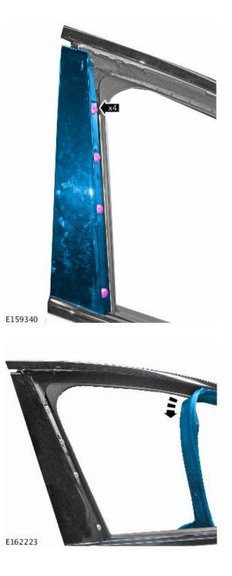
**21.** Using soapy water, install the margin seal.
