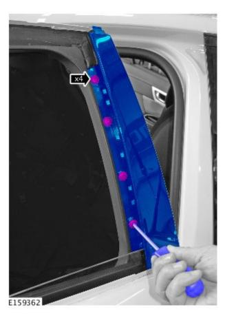
**48.** Apply protective tape to the existing trim prior to fitting the new door C-pillar trim.
