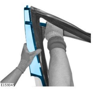
**16.** Install seal to the new door B-pillar.
