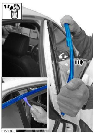
**36.** Remove the door C-pillar fixing.
