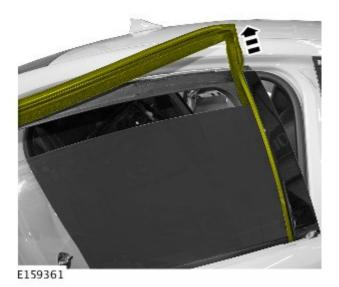
**40.** Displace the rear glass to gain access to door C-pillar fixing (see TOPIx Workshop Manual, Section 501-11).
