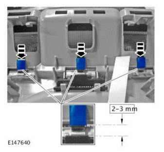
7. NOTE: Do not damage the printed circuit board.
