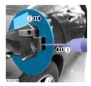
4. Using a suitable tool, release the retaining clips and
