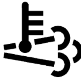
High Exhaust System Temperature (HEST)
