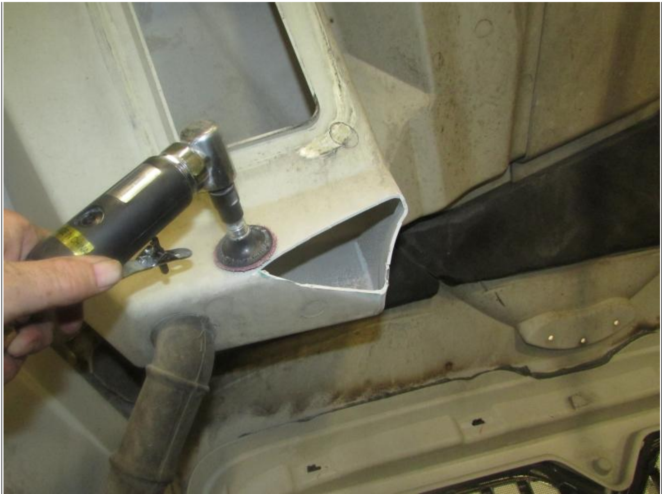
Figure 8: Sanding/roughing of the patch area.
