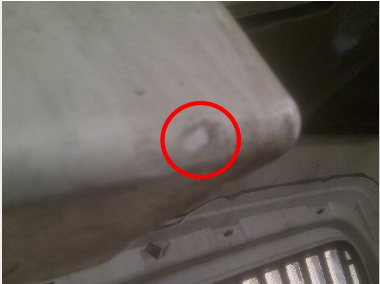
Figure 2: Rub mark in the hood from CACOT sensor contact (air inlet cowl).
