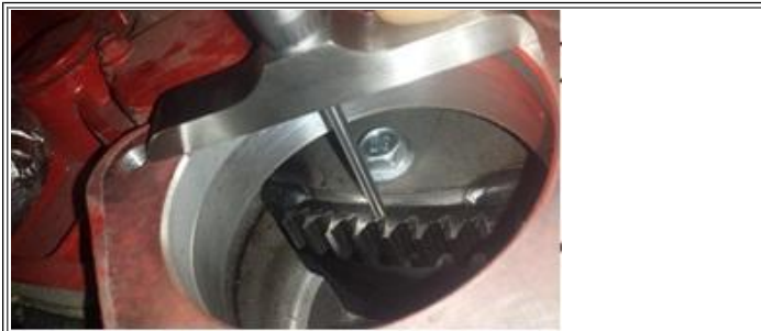
Figure 2: Starter Mount Face to Ring Gear Face Measurement
