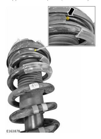
**3.** Using a suitable marker, make an alignment mark through the spring, packer and shock absorber.
