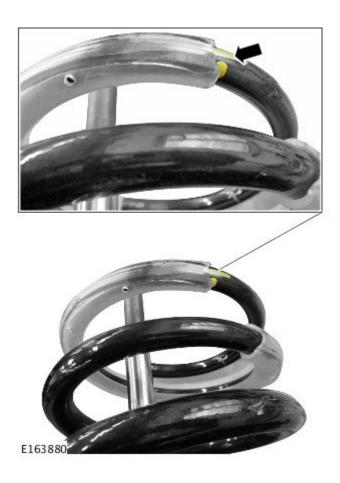
7. NOTE: During assembly, make sure that the alignment marks line up.
