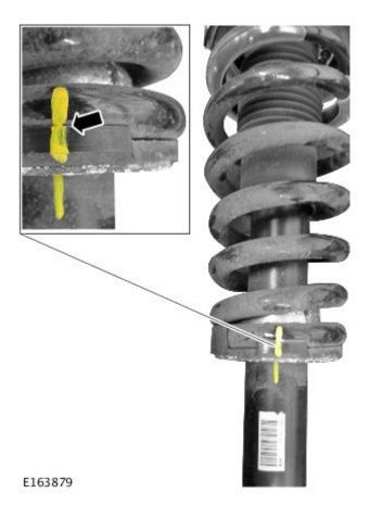
8. NOTE: Make sure the spring assembly is located in the top mount correctly.
