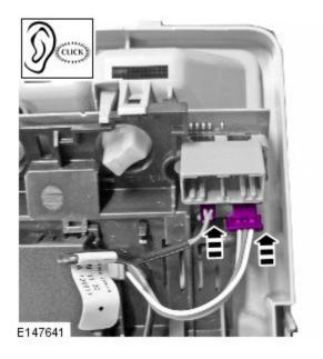
10. Install the front overhead console lamp assembly (see TOPIx Workshop Manual, section 501-12).
