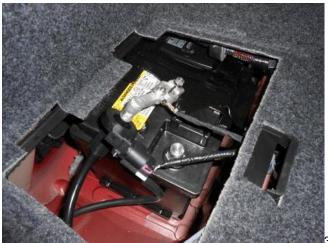
3. Position the vehicle in a stall with a hoist and disconnect the negative battery cable. Refer to *Battery Negative Cable Disconnection and Connection* in SI.
