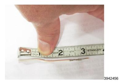
5. Cut off approximately 76 mm (3.0 in) of the end of the tin plated terminal
