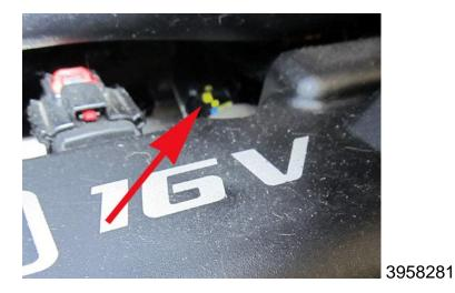
2. Using a medium depth 24mm socket, remove (unscrew) the PCV valve and seal from the camshaft cover.
