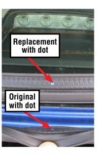
**STEP 3:** After the trunk stoppers (and weatherstrip on STI models ONLY) have been installed, close the trunk lid while paying close attention to the points listed below.
