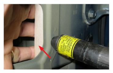
Another area which may be the source of these sounds is shown in the photos below. Although the right fender is removed in the photo, the structures are symmetrical side to side. Separate the layers of sheet metal using a flat-blade screwdriver but use caution not to tear or separate any spot welds.
