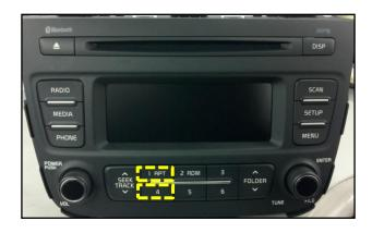
13. To access the Engineering Mode on Rio (UB) vehicles: Press and hold buttons 1 and 5 simultaneously for 2 seconds, then, press the button 1 four times in quick succession.
