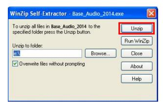
8. Unzip the downloaded file directly to the root directory of the USB flash drive being used for the update.
