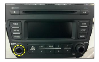
12. To access the Engineering Mode on Sorento (XMa) vehicles: Press and hold buttons 1 and 4 simultaneously for 2 seconds, then, press the button 1 four times in quick succession.
