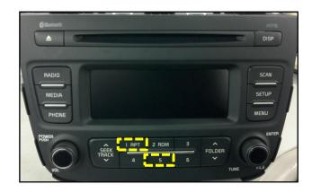
14. Once in engineering Mode, the system will display the software version on the screen. Confirm the original software version matches the information shown in the table below.
