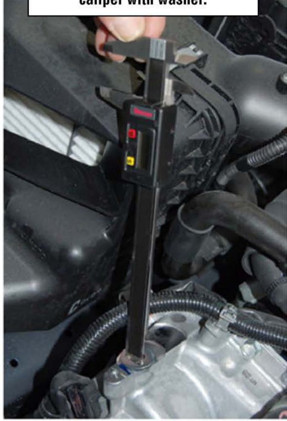
Measurement taken using digital caliper with washer.
