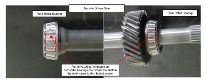
**IMPORTANT:** If the transfer driven shaft bearings are damaged or failed, **thoroughly** clean and inspect all the internal components of the transmission before reassembly. In very severe cases where metal contamination damage is extensive, transmission assembly replacement may be required. If within the warranty coverage period, completion of an Assembly Repair vs. Replacement worksheet is required.
