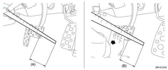
The specification for pedal stroke to activate the BLS is 5.5mm +/- 2.5mm (>3mm but <8mm).
