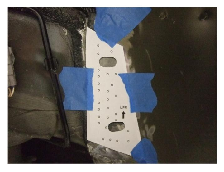
The punch tester will be used to make indentations at all of the 27 spots.
