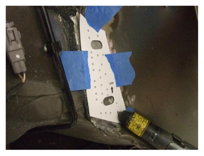
9. Remove the template. The punch tester makes a 1.8mm indentation.
