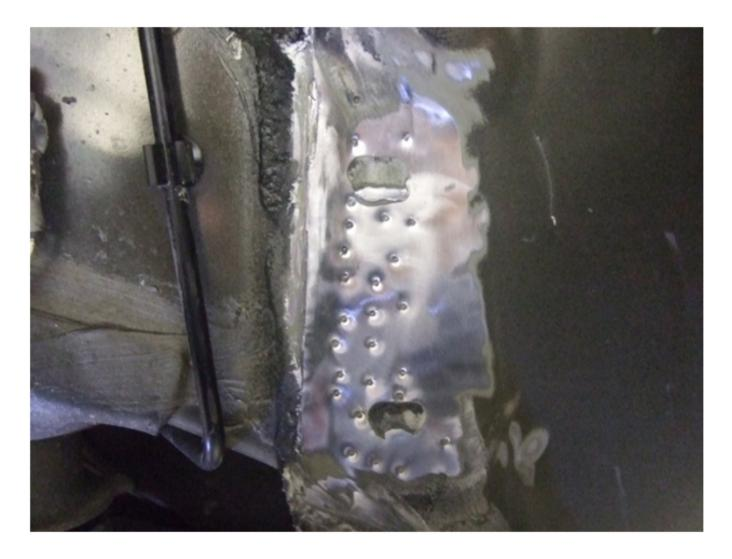
The indentations need to be increased to 3mm using a Snap-on Center Punch 3/16" point, 6" (stock # PPC4A) or equivalent.
