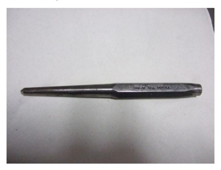
10. Using a 3/16 tapered punch and hammer, increase each indentation to 3mm.
