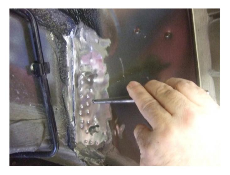
Measure to insure that a 3mm indentation was made using the punch. **NOTE:** This is a critical step; make sure each indentation measures 3mm.
