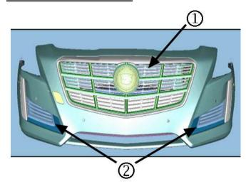
**Note:** For vehicles with bright chrome grille kits, replace the upper grille (1) and front outer grilles and bezels (2) with the black chrome service parts noted above. For vehicles with black chrome grille kits, replace ONLY the front outer grilles and bezels (2) with the service parts noted above.
