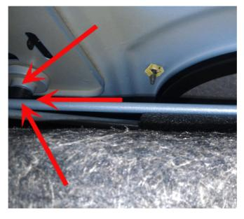
4. Add felt onto the package shelf trim opening to prevent movement between the trim and the child seat tether cover if the felt is not present. Use Kent Adhesive Backed Flocking Tape p/n KT13295 or equivalent see pictures below.
