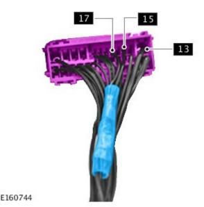
**6.** If necessary, repeat step 5 to the front left door electrical connector (C3A-C2).
