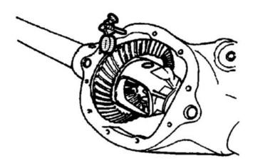
2. Install the J-25025 pins and the J-8001 indicator to the axle housing.
