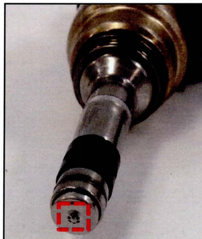
New injector showing location of Spray Orifices
