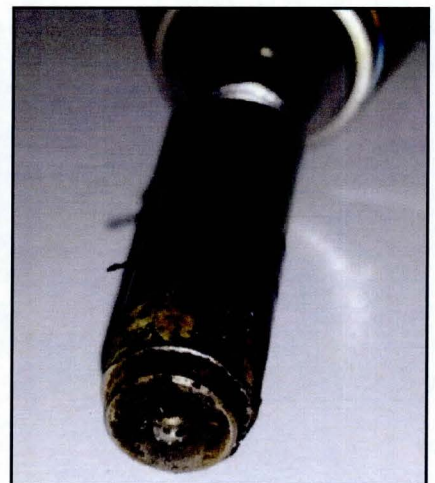
Normal injector appearance while in service
