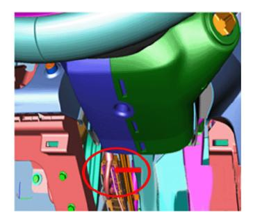
2.2. Visually inspect the I/P Harness BCM Connector 19151262 Cavity 14.
