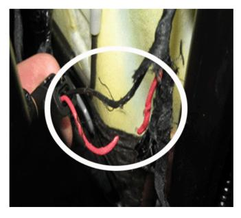
This condition may be caused when the lead screw on the up/down motor (1) comes in contact with the haptic pigtail (2) and cuts through the pigtail wire as shown in the illustrations above.
