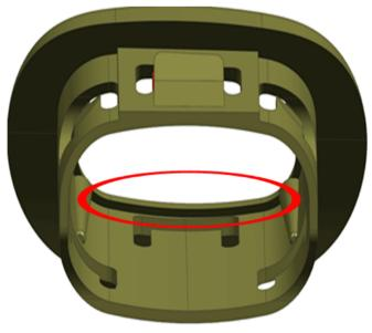
This may be due to the locking tab hanging up on the lip inside the bezel, shown in the illustrations above, and not allowing the door lock knob to move upward and unlock the door.
