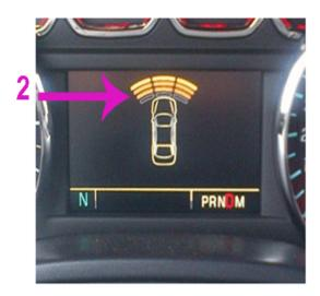
The vehicle may have an instrument cluster parking assist display with bars that show "distance to object" and object location information for the Rear Park Assist (1), and on some vehicles, for the Front Park Assist (2). As the object gets closer, more bars light up.
