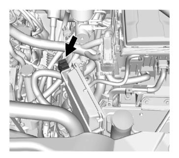
The bi-fuel system has two fuses that are part of the engine compartment wiring harness. Both fuses are in a plastic holder that is mounted inside the engine compartment, near the accessory battery tray.
