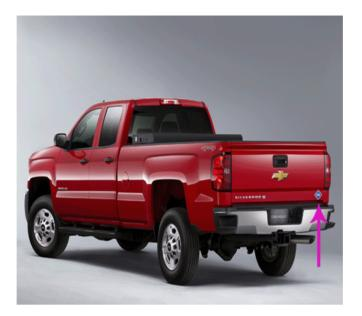
There is an identifying blue diamond-shaped CNG label on the rear of the vehicle. Do not remove this label. This label is necessary for compliance with NFPA-52 regulations. Driving without this label may violate the laws or regulations in some states. Replacement labels can be ordered from your Dealer.
