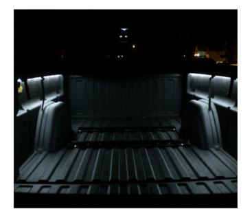
The cargo lamp provides more light in the cargo area of the vehicle, if needed. The LED under rail lights inside of the pickup box also turn **ON**, if equipped.
