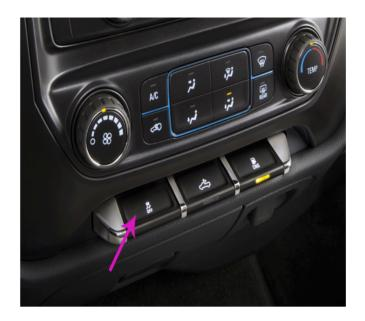
The vehicles have a Traction Control System (TCS) and StabiliTrak<sup>®</sup>, an electronic stability control system. These systems help limit wheel spin and assist the driver in maintaining control, especially on slippery road conditions. Both systems come **ON** automatically when the vehicle is started and begins to move. The systems may be heard or felt while they are operating or while performing diagnostic checks. This is normal and does not mean there is a problem with the vehicle.
