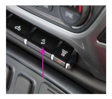
If equipped, HDC can be used when driving downhill. It sets and maintains vehicle speed while descending a very steep incline in a forward or reverse gear. The HDC switch (1) is on the center stack, below the climate controls. Press the HDC switch (1) to enable or disable HDC. Vehicle speed must be less than 31 mph (50 km/h). The HDC light displays on the instrument cluster when enabled.
