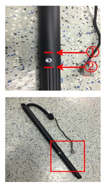
**Note:** The screw will hold the strut together for removal.
