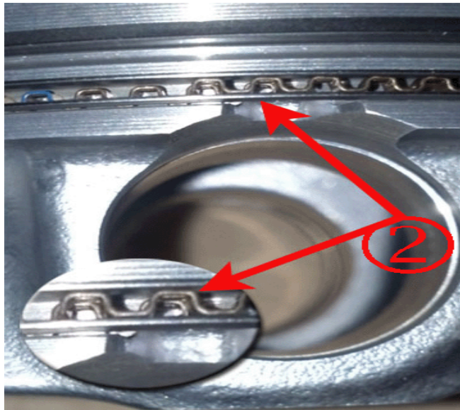
Example of improperly positioned oil control expander ring. (Overlapped).
