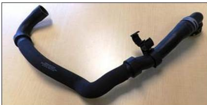
New coolant hose 5N0121051M with new double hose retainer.
