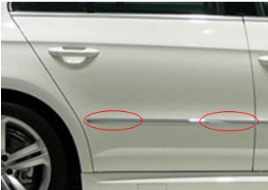
Figure 1 (the red ellipses show the area which can be affected by the corrosion)
