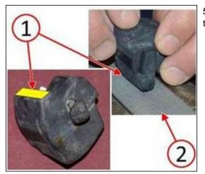
5. Using a coarse file (2), remove 1 mm of material from the rubber bumper surface (1) indicated in (Fig. 2).
