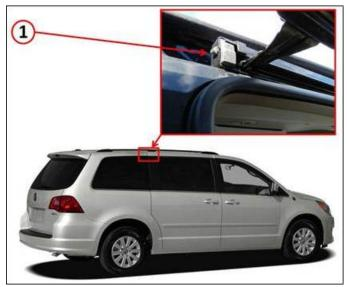
3. Open the right rear sliding door, remove the rubber bumper (Fig. 1) from the rear end of the upper door track and <u>close the door</u>.
